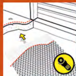
8 Cutting Alveplac® to shape.
