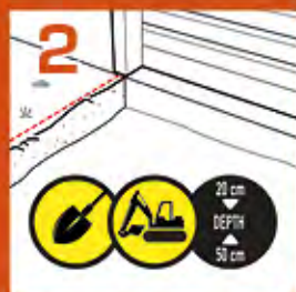
2 Prepare the ground.
