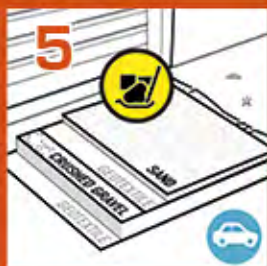
5 Lay the sub-base for traffic areas.
