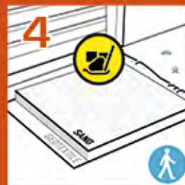
4 Lay the sub-base for pedestrian areas.
