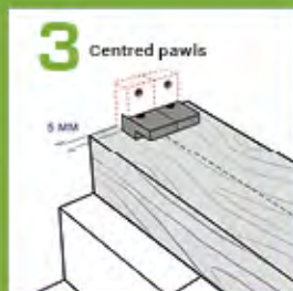
3 Begin laying the decking.
