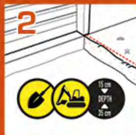
2 Prepare the ground.
