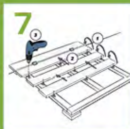
7 Turn, slide and fix each decking board.
