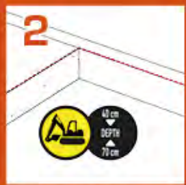
2 Prepare the ground.
